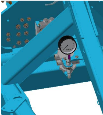
Picture 16 Cutting cylinder safety pressure gauge
